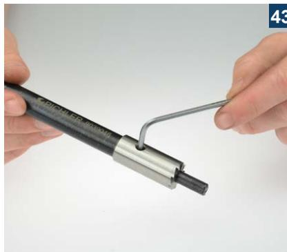
Slide it flush on to the basic device and make sure, that it's clamped on the flat spot of the basic device.
