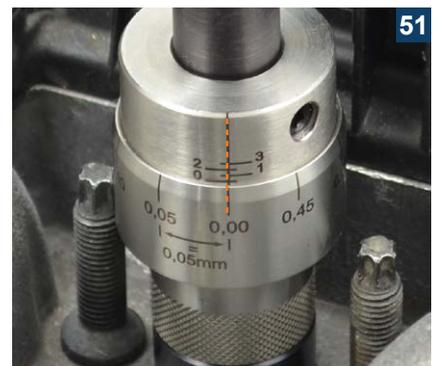
Push the injector seat milling cutter all the way in, press the depth stop on the centring cone and at the same time clamp the upper scale ring.
