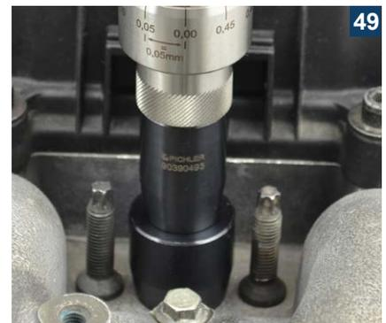
Retain the upper scale ring and turn the lower ring on the depth stop so long in a **clockwise direction**, until the stop. **50**
