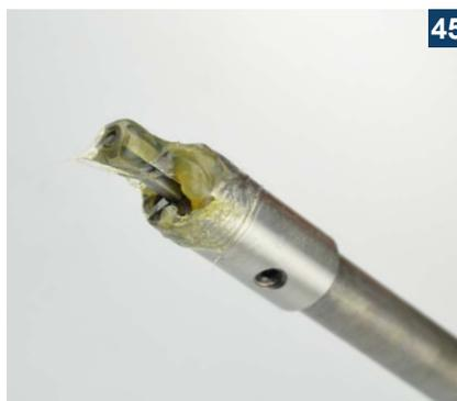
To bond the chips and for a better cutting result, immerse the milling cutter slightly rotating clockwise into the cutting grease.
