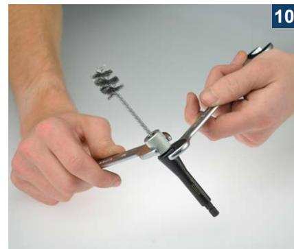
Insert the brush holder into the flexible shaft, clamp the shaft in an electrical drill and place the brush in the injector shaft.
