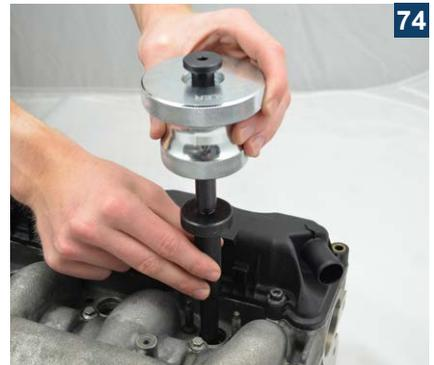
Tap gently with the slide hammer the extractor claw of the sealing ring extractor into the bore of the sealing ring.
