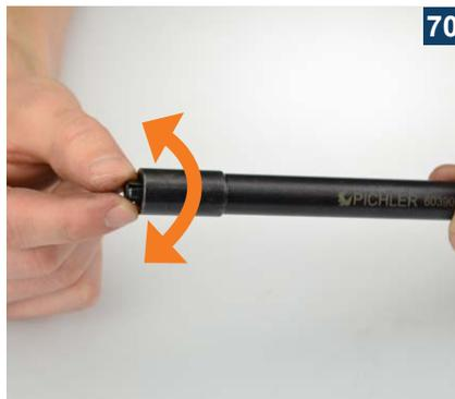
Use a new sealing ring and place it on the extraction claw in order to adjust the grip depth.
